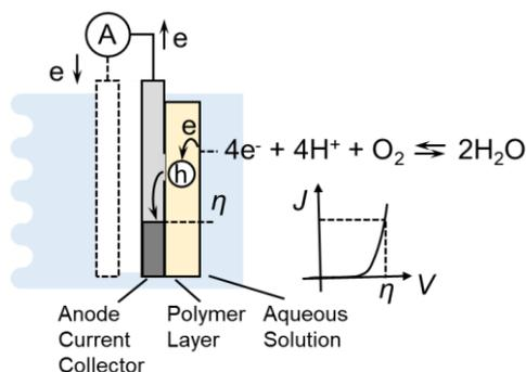
Figure 1. Energy-level diagram for the polymer-modified anode and water oxidation/oxygen evolution reaction and current density ( $J$ ) curve for the oxygen evolution reaction;  $\eta$  is the overpotential to achieve the  $J$
