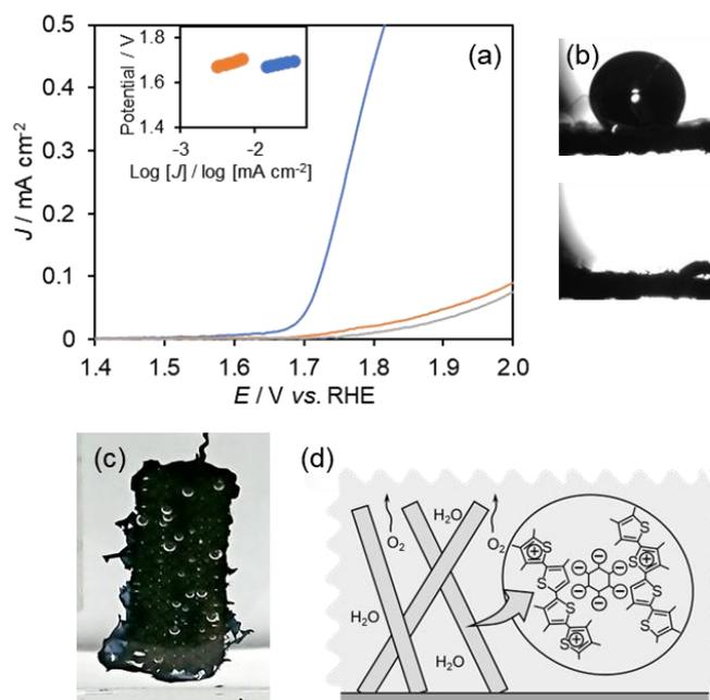
Figure 4. Water oxidation performance: (a) the anodic  $J$  and (inset) Tafel slope of the PEDOT-PA/pHEMA complex (blue), and PEDOT/pHEMA (red), and CC (gray), (b) Contact angle of (upper) CC substrate and (lower) PEDOT-PA/pHEMA-modified CC, (c) the PEDOT-PA/pHEMA complex during the anodic operation, and (d) Schematic image of the PEDOT-PA/pHEMA complex
