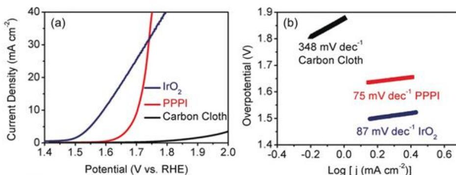
Figure 3. Water oxidation performance: (a) the anodic  $J$  and (b) Tafel slope of the poly(phenylene pyromellitic diimide) (PPPI)/CC and the benchmark  $\text{IrO}_2$  (Copyright from Wiley-VCH 2018: Ref. 26))
